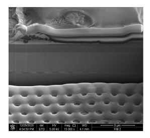
74. The composite image above shows an n-type semiconductor layer having a surface, and a mesa located over a first portion of the surface of the n-type semiconductor layer, a first n-type metallic contact layer located over at least a
