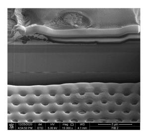
67. The composite image above shows an n-type semiconductor layer having a surface, and a mesa located over a first portion of the surface of the n-type semiconductor layer, a first n-type metallic contact layer located over at least a portion of the n-type contact region in proximity of the mesa boundary and a second n-type metallic contact layer located over a second portion of the n-type
