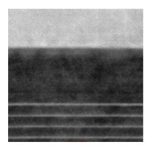
109. As shown in the TEM images above, the semiconductor heterostructure includes an active region, and a group III nitride semiconductor layer located between the active region, and the semiconductor layer including a plurality of inhomogeneous regions.
