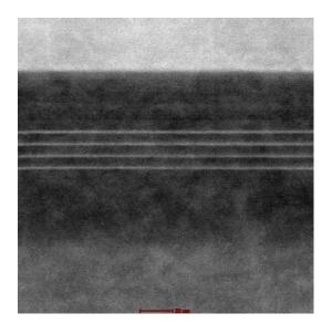
84. Below is a SEM image taken after a hole was milled into the LED chip using a FIB. The FIB-SEM image shows at least one contact over the active layer and adjacent to the composite layer.
