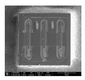
59. Two metallic contacts are deposited on the surface of the UV LED's semiconductor structure, as shown in the SEM image below. One of these contacts in the LTPL-G35UV275GC-E UV LED comprises at least two corners.
