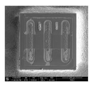
73. Below is a SEM image taken after a hole was milled into the LED chip using a FIB.
