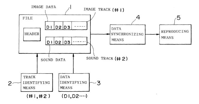
The image and sound data in the file (1) are identified as separate tracks (#1 and #2). (*Id.*, 1:59-62.) Further, each unit time (e.g., 1 second) of the audio and video tracks are separately identified (**D1**, **D2**, **D3**, etc.). (*Id.*, 1:62-65.) Header information in the file can be used to synchronously reproduce the unit times of the image and sound data. (*Id.*, 1:66-2:4.)
