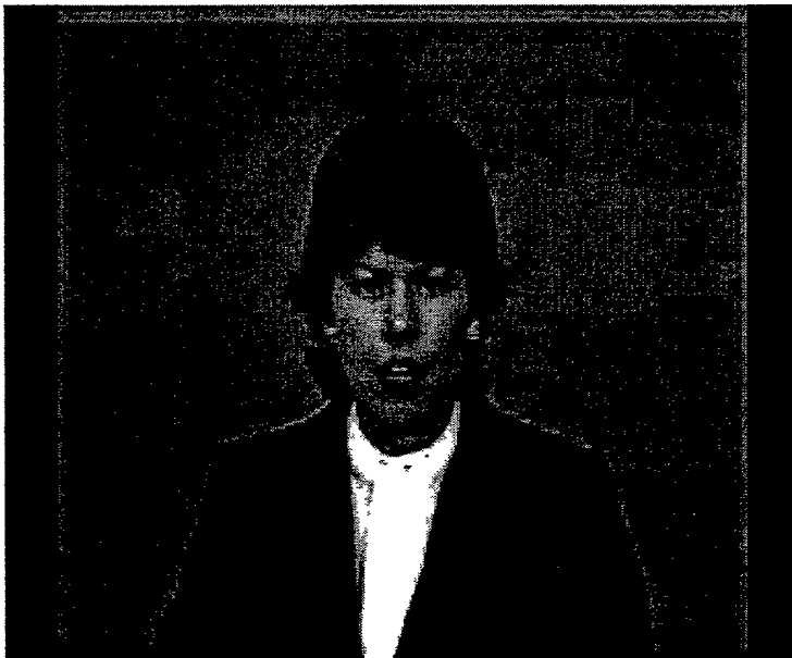
Figure 16 "Claire" I frame from the MPEG-1 coder, \Delta_G=1.3 , PSNR=37.5dB, compression ratio=26.7:1
