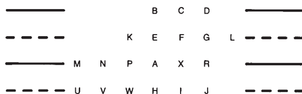
Fig. 6.2.3 Pel configuration for NTSC composite color TV signal sampled at four times color subcarrier frequency. Pels K , L , M , I and U have the same color subcarrier phase as pel X .
