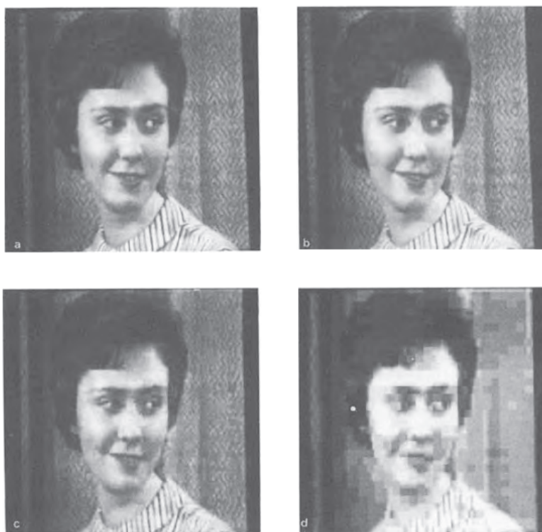
Fig. 5.3.25 Coded image "Karen" using the separable 2D-DCT with 8 \times 8 blocks, uniform quantization and entropy coding. The coefficients having the largest MSV are sent. PSNR's and entropies are (left-right, top-bottom): (a) PSNR = 38.0dB, 1.24 bits/pel (b) PSNR = 33.5dB, 0.67 bits/pel (c) PSNR = 29.9dB, 0.36 bits/pel (d) PSNR = 25.7dB, 0.13 bits/pel
