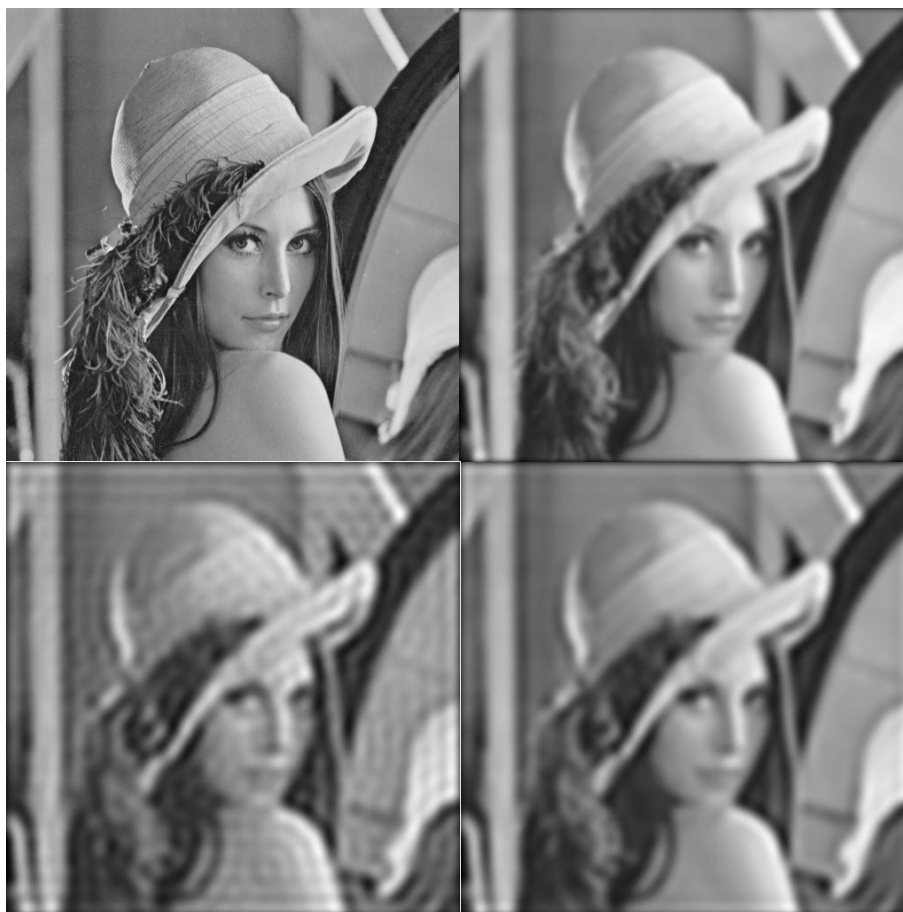
Figure 13: Plots of the original lena image (top left image) along with lowpass filtered versions using a Gaussian filter (top right image), an ideal filter (bottom left image) and a Butterworth 4-th order filter (lower right image). The cutoff frequencies for all lowpass filters was 50.
