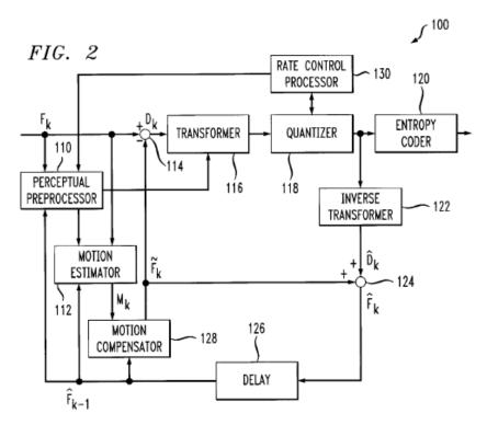
Figure 2 is a block diagram of video encoder 100. *Id.* at 5:32–33, 7:53–55. Video encoder 100 includes perceptual preprocessor 110, motion estimator 112, and signal subtractor 114 coupled to the input of encoder 100. *Id.* at 7:63–67. Motion estimator 112 is also coupled to perceptual preprocessor 110. *Id.* at 7:67–8:1. Encoder 100 also includes
