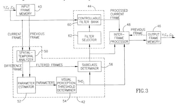
Figure 3 is a block diagram illustration of a visual lossless syntactic encoder. Ex. 1001, 4:36–37. The encoder comprises input frame memory 40, frame analyzer 42, intra-frame processor 44, output frame memory 46, and interframe processor 48. *Id.* at 5:67–6:3. Frame analyzer 42 comprises spatial-temporal analyzer 50, parameter estimator 52, visual perception threshold determiner 54, and subclass determiner 56. *Id.* at 6:22–24.
