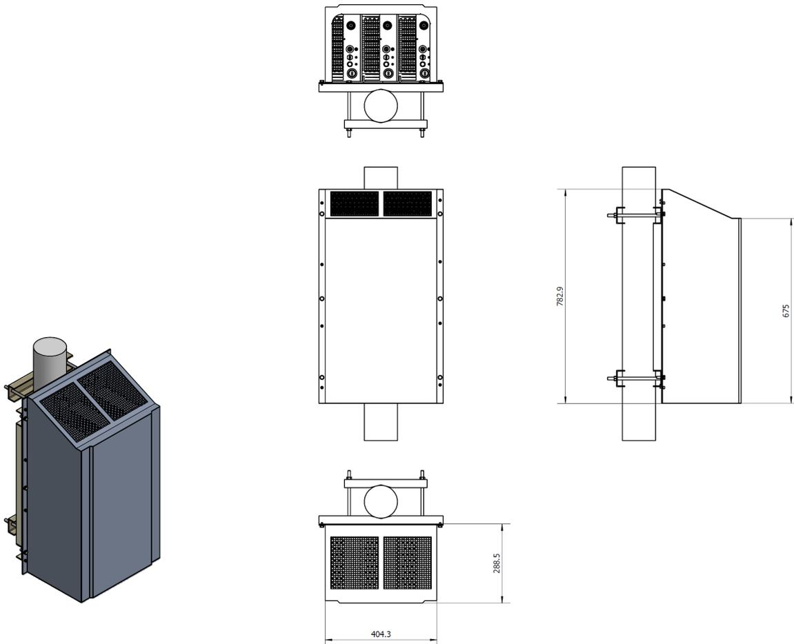
**Figure 2-5. 3 Remote Unit Assembly With Solar Shell**
