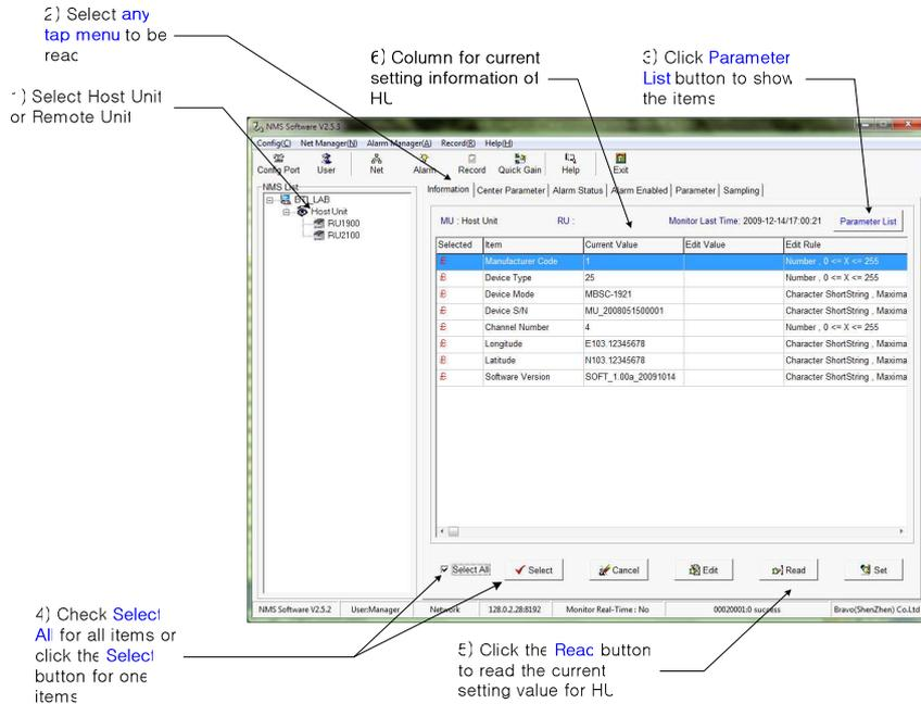
**Figure 3-12. Read the current setting for the system**
