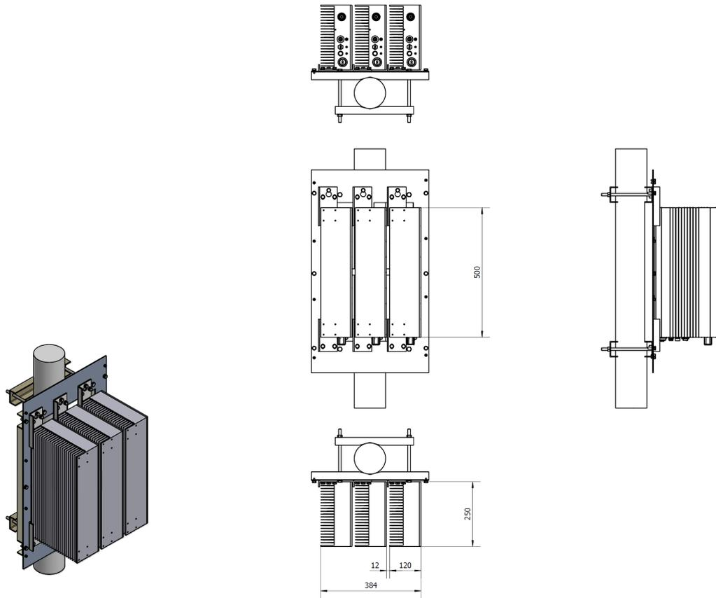
**Figure 2-4. 3 Remote Unit Assembly Without Solar Shell**
