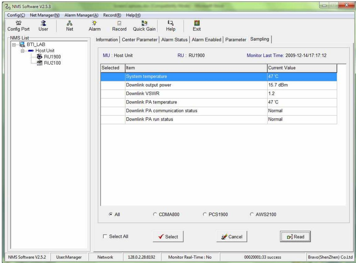
Figure 3-17. Check the system performance
