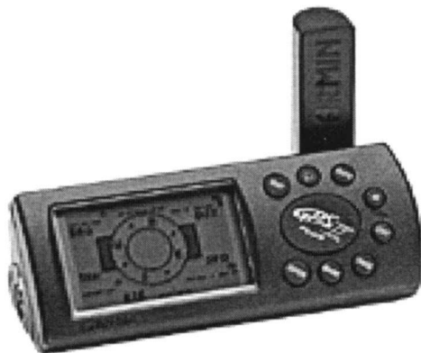
Fig. 4. Portable GPS receiver by Garmin.
