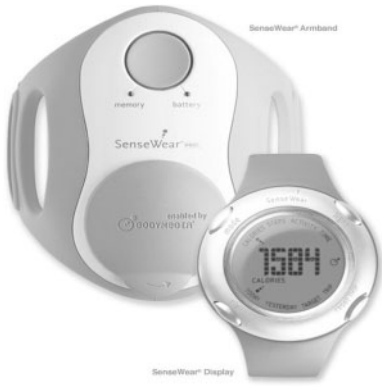
Figure 8 SenseWear Pro3 Armband, worn on the upper arm.
