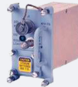
KIV-78 IFF Cryptographic Computer
