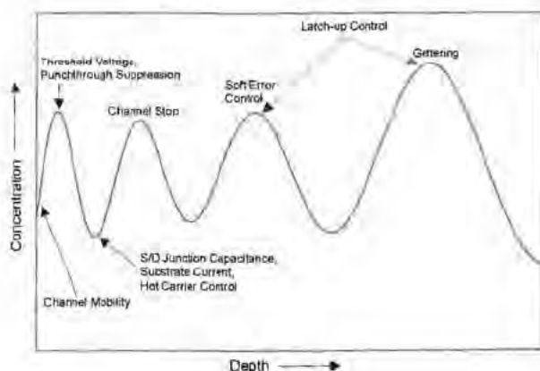
Figure 11 Doping profile of a modulated retrograde well structure, showing the device parameters affected by the doping level at each depth. Adapted from references [40,41].
