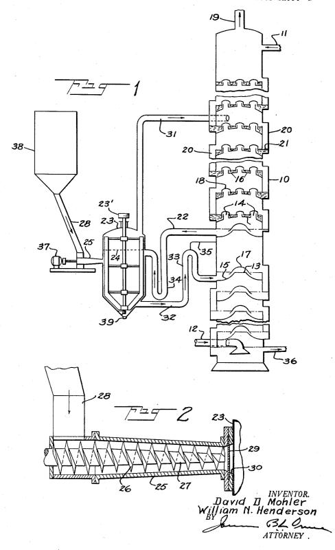
PROCESS AND APPARATUS FOR DRY LIME TREATMENT OF LIQUORS
