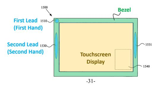
193. Multiple scenarios may be envisioned for the user to contact these electrodes, such as in a portrait orientation where both hands are at the bottom of the touch display, providing an ECG reading with an adjacent first hand and second hand on electrodes 1510 and 1530, or a first hand may be positioned on lead 1510 while a second hand touches a power button near lead 1530.
