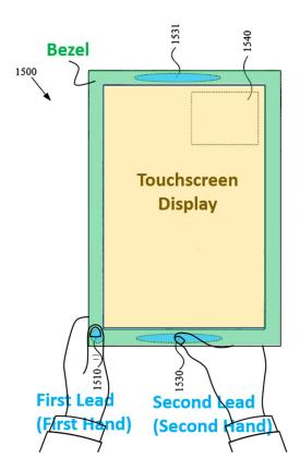
194. Further, since this claim is an apparatus claim, the electrodes need only be capable of a configuration where different hands touch electrodes 1510 and 1530. Finally, Markel teaches that "one or more electrodes may be disposed in any of a variety of locations on the MCD." EX1005, [0052].
