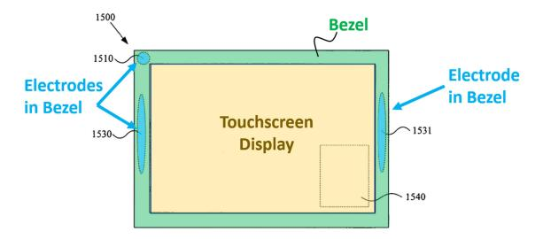
164. The embodiments in Figure 1 and 15 both have touchscreens, as I explain in this section, with bezels or borders surrounding the touchscreens, as illustrated below. Moreover, a POSITA would have understood that the locations of the electrodes in display device 140 could be the same as the electrode locations shown in Figure 15.
