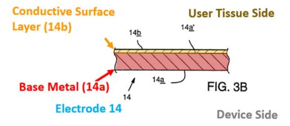
EX1006, Fig. 3B (rotated). Mills's electrode 16 has the same structure as 14, with plating on the outside. EX1006, 2:16-20, 4:10-13.
