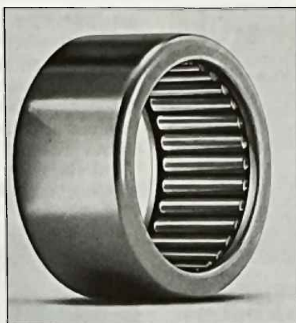
Fig. 2-14 — Grease-retained, drawn-cup needle roller bearing has a slightly higher load rating than a mechanically retained bearing.
