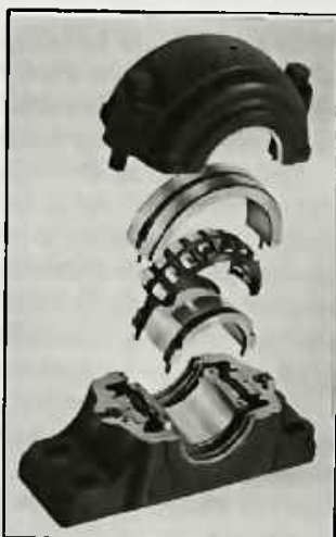
Fig. 2-25 — Split spherical roller bearing enables easy replacement without disturbing other components.
