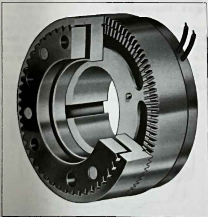
Fig. 5-8 — Multiple-tooth clutch (stationary field).
