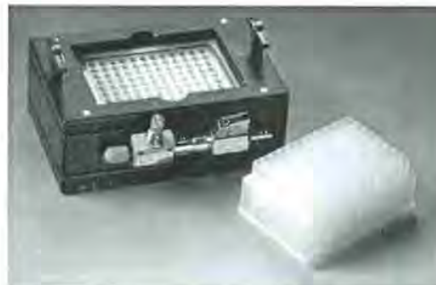
Fig. 2: GeneSys - 1 shown with Prep-Sep manifold™ and 96 well extraction plate.
