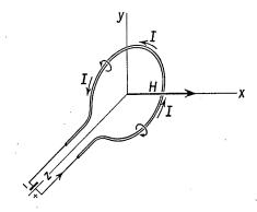
is in a straight portion of the wire, then, if we imagine the thumb of the right hand to be placed along the wire and pointing in the direction of the current, the curled fingers of the right hand will point in the direction of
