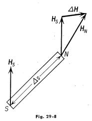
in Figure 29-8, where  $\Delta \mathbf{H}$  is the vector difference between the fields at these two poles. The net force on the magnet is due to the change in the field  $p \Delta \mathbf{H}$ , for if p is the pole strength of the magnet, the force on the magnet is
