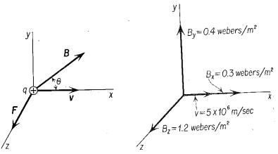
Fig. 31-1 The force  $\mathbf{F}$  exerted on a charge q moving with velocity  $\mathbf{v}$  in a magnetic field of induction  $\mathbf{B}$ .  $\mathbf{B}$  and  $\mathbf{v}$  are in the x-y plane;  $\mathbf{F}$  is along the z axis.
