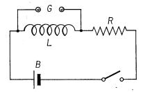
Fig. 32-14 A spark-gap G placed across the terminals of an inductor.
