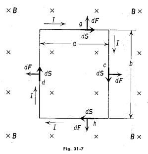
The force on each side b of the coil is given by Equation (31-11) as
