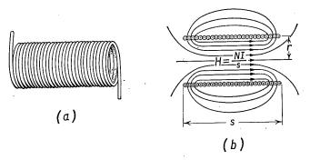
Fig. 30-11 (a) Windings of a solenoid. (b) Magnetic field intensity inside a solenoid. Current is coming out of the wires on top and going into the wires on bottom.
