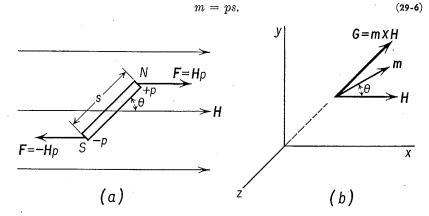
Fig. 29-7 (a) Forces on a bar magnet in a uniform magnetic field. The plane of the paper is the x-y plane. (b) When the magnetic moment vector m and the magnetic field H lie in the x-y plane as shown, the torque G on the magnet is parallel to the z axis.
