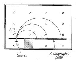
Fig. 31-3 Beta-ray spectrometer:
