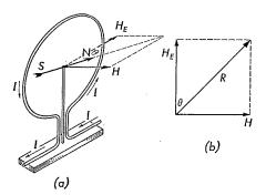
Fig. 30-9 (a) Tangent galvanometer. The plane of the circular coil is parallel to the earth's magnetic field. (b) The two magnetic fields which act on the N-pole of the small compass needle.  $H_E$  is the horizontal component of the earth's magnetic field; H is the intensity of the magnetic field produced by the current. R is the resultant of these two field intensities.  $H = H_E \tan \theta$ .
