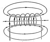
Fig. 30-5 Magnetic field due to a current in a long cylindrical coil or helix.
