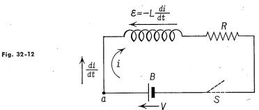
is in the clockwise direction, as shown in the figure, and that the current is increasing so that the direction of the rate of change of current is in the same direction as the current itself. Starting at the point a and applying Kirchhoff's laws by moving a probe charge around the circuit in the direction of the current, we find
