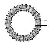
in the form of a ring. The magnetic field intensity within the toroid is given by Equation (30-5), where s now represents the mean circumference of the ring, shown in Figure 30-12.
