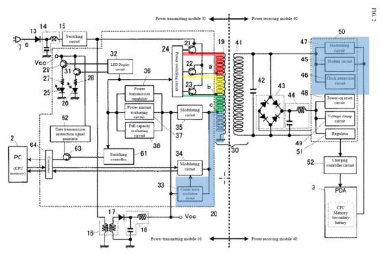
Prelim. Resp. 46. Figure 2 of Okada is a block diagram illustrating the electrical configuration of the common charger cradle 4 equipped with power transmitting module 10 and the PDA device being charged equipped with the power receiving module 40. Ex. 1005 ¶ 37. As described by Patent Owner, Okada uses the blue portion of the coil—from tap "c"—to send a communication carrier wave, receive an information signal from the
