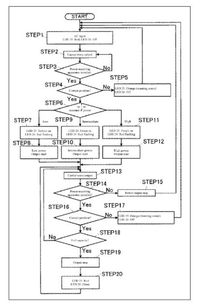
Prelim. Resp. 39. Figure 3 above is a flowchart showing the operations carried out in Okada between power transmitting module 10 in Figure 2 and power receiving module 40. *Id.* at 38.8
