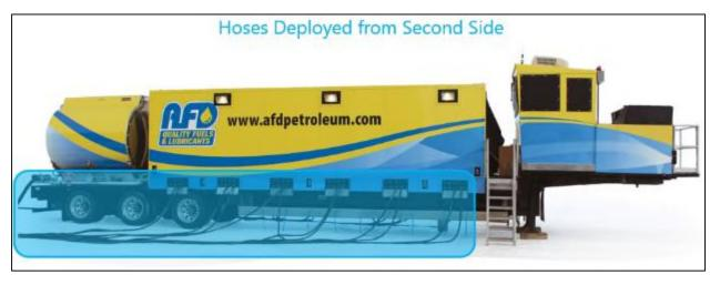
In the second image, 12 hoses are deployed on the near side. *See id. AFD* describes that there are 24 hoses in total: "The main body of the trailer contains 24 fuel reels, each with 300 - 450" of 1" hose ...." hose ...." hose 355, thus a POSITA would have understood
