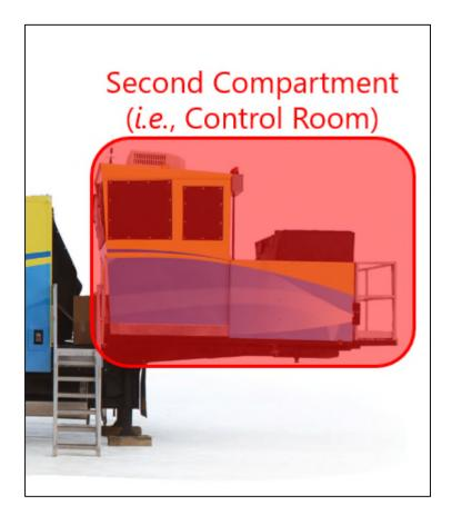
286. A POSITA would have understood that this compartment is the control room at least because a POSITA would recognize the necessity of separating the control room from the main compartment in order to reduce the area classification of the control room from Class I Div. 2 to unclassified, and to allow the use of
