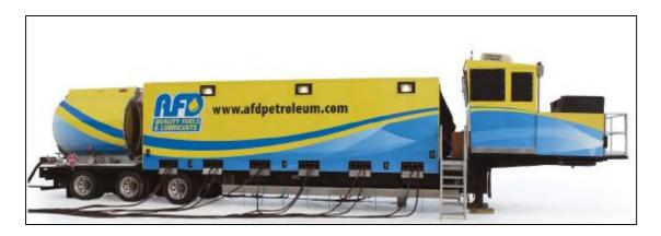
129. The AFD Onsite Refueling System includes a trailer having a main compartment having 24 fuel reels, 24 hoses, a 10,000 L fuel tank. According to AFD, "The main fuel tank has an internal pump to attach to an alternative fuel source in
