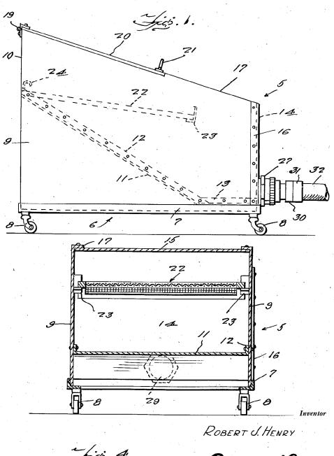
AIRPLANE FUEL TANK DRAINING AND TRANSFERRING DEVICE
