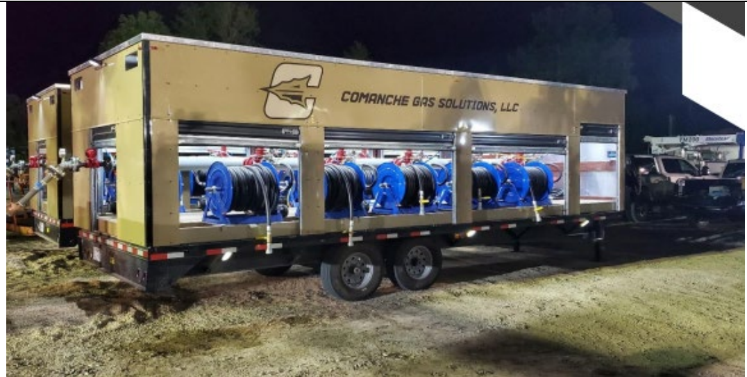
“The AFS has 27 hose reels per unit to accommodate horsepower”
