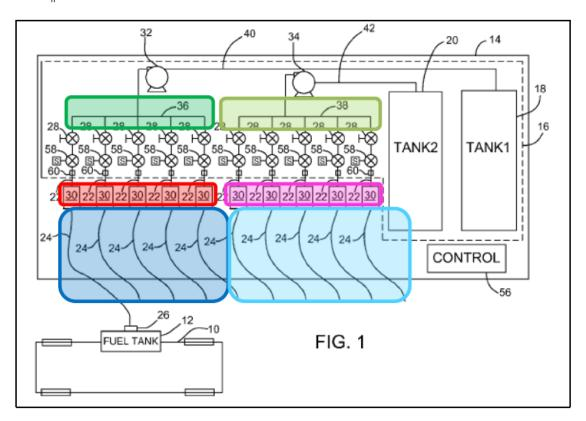
As shown above, Van Vliet's equipment includes a first manifold 36 connected to a first group of hoses 24 (dark blue) and hose reels 30 (red) and a second manifold 38 connected to a second group of hoses 24 (light blue) and hose reels 30 (pink). Hose reels 30 are arranged parallel with the sidewalls of the trailer, and hoses 24 are deployed through openings in the trailer's sidewalls. *Id.*  $\P$ ¶ 15, 24.
