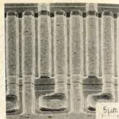
Fig. 8. SEM micrograph showing some of the electrodes of a linear CCD sensor. The average width of the gaps between the electrodes is 1\text{ }\mu\text{m} . The thickness of the Al/Si electrodes is 0.8\text{ }\mu\text{m} .
