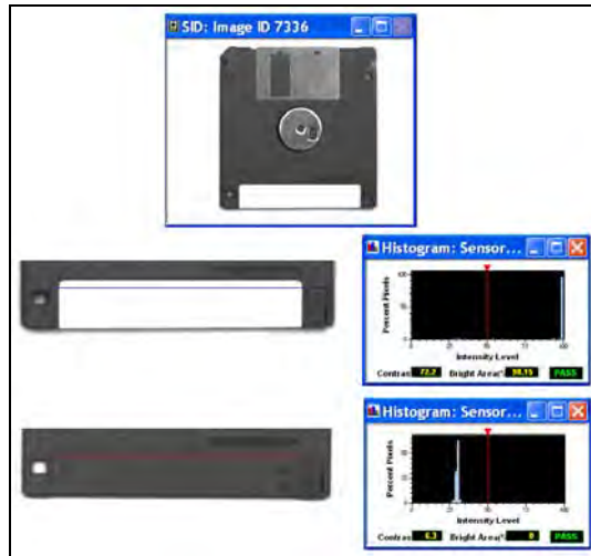
Figure 3-5: Use of an Intensity SoftSensor to verify the presence and correct position of a label
