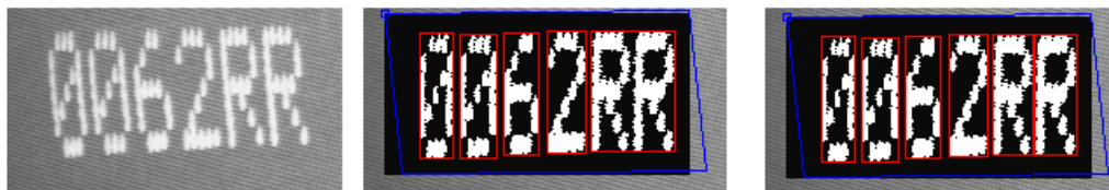
Figure 3-24: Use of the extraction tools to separate individual characters.
