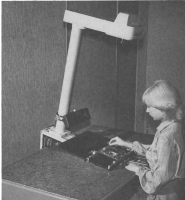
Figure 10.5 A light guided component location – by projected light beam
