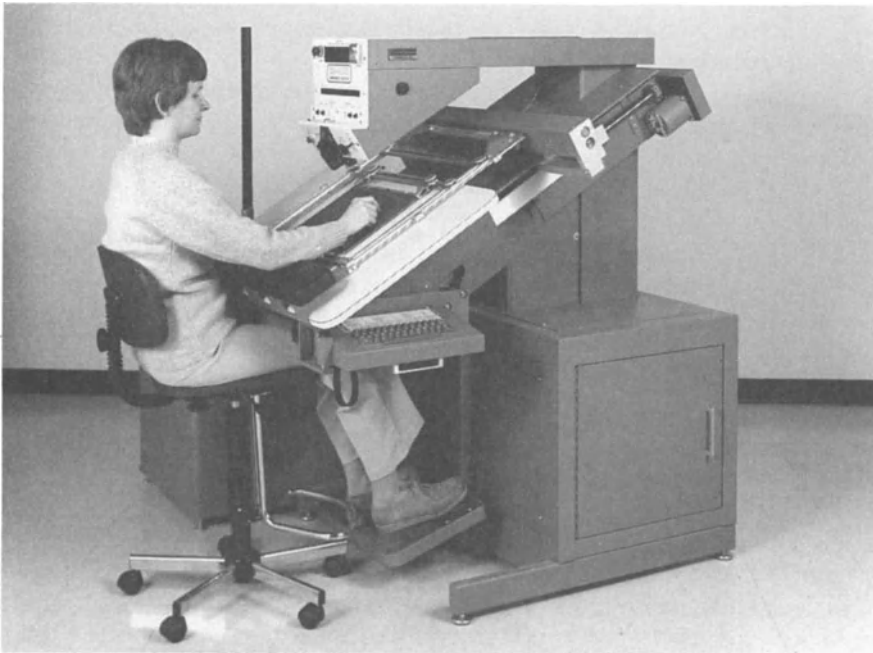
Figure 10.6 A light guided station (Contax) including an out and clinch mechanism sophistication. In the early days use was made of 35 mm film, slides, or various plates in order to produce the image. This was subsequently replaced by a single projected beam of light which was manipulated so as to produce a single or multiple image on the pcb under computer control, the light beam being deflected by galvanometer mirrors and therefore apparently static to the operator. A sophisticated improvement on this has been to replace the illuminator with a laser, thus increasing the apparent brightness of the image on the pcb and simplifying the optics necessary to increase that brightness. Figures 10.4, 10.5 and 10.6 show such workbenches.
