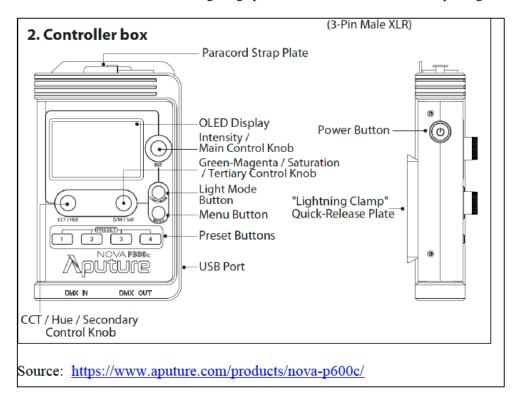
70. The '258 Accused Products include a controller comprising an input interface for receiving user input to enable a user to select user customisable cinematic lighting special effect from said range of different user customisable cinematic lighting special effects:
