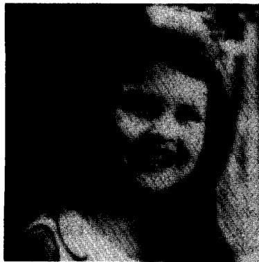
Fig. 3. Unprocessed output of 128 \times 128 CMOS active pixel sensor.
