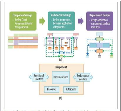
Figure 2. Cloud Component Model (CCM)-based development: (a) design methodology, which comprises component, architecture, and deployment design; and (b) CCM component architecture. CCM's component-based approach is suitable for both Web-based and mobile applications.
