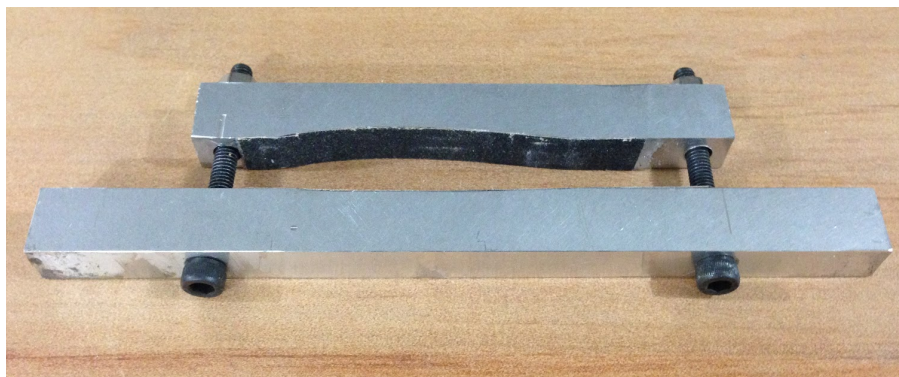
Figure 3: Part clamping fixture showing sandpaper adhered to airfoil geometry
