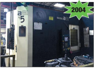
Makino mod. A81 Horizontal CNC Machine Center
