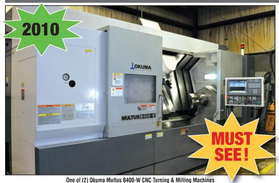
(2010) Okuma mod. MULTUS B400-W, 7-Axis CNC Turning and Milling Machine w/Okuma OSP-P200L CNC Controls, Single Spindle w/Subspindle, Knuckle Joint Head, 3-Jaw Chuck, Auto Tool Changer, Hakusan Chip Conveyor, Chip Blaster, High Pressure Coolant System, 12"/15" Chucks. S/N 151177
